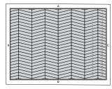
14. Build the final column using the same placement order, beginning near wall A and finishing near wall D. Measure, mark, and cut the fill pieces at walls C followed by cutting fill
