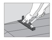
11. Measure, mark, and cut pieces near wall A. These cuts will be installed by positioning the long groove edges into the long tongue edges. If necessary, use a pull bar to lock the long edges together for the fill pieces at the walls. (Note - A pull bar should only be used against the cut edges and never against the plank edges/profiles.)
