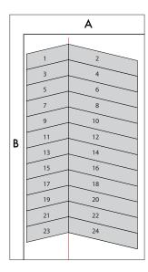
10. Continue forming the V column. Ensure the center of the V column is always aligned with the starting line. Install planks and maintain joint alignment until no additional full pieces can be installed within the V column.
